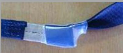
Attach the reserve parachute bridle to the center of the harness bridle using a larks head knot, sealed with a heat shrink tube to keep it in place.
