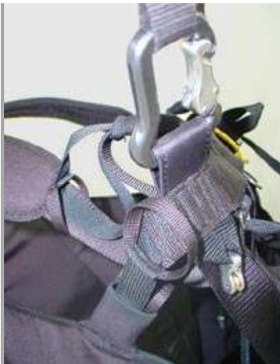
2. The **Back/Side Strap** Adjusters these are similar to previous Apco Harnesses. They are best adjusted while the harness is suspended from a suitable structure, before the first flight is made.
