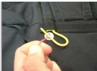
Tighten the pull cords so that the nylon closing loops are protruding through the grommets and push one of the locking cables through one of the closing loops.
