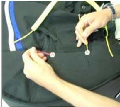
Next close flap No.4 over flaps No.3, No.2 and No.1. Thread the pull cords through the grommet attached to flap No.4.
