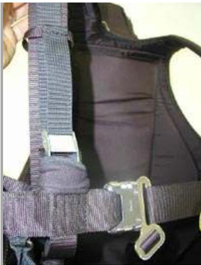
1. The **Shoulder Strap** Adjusters are similar to most Apco Harnesses, differing only in the minor improvement, which prevents the free ends of the adjustment webbing from flapping around in the wind. These straps are best adjusted when standing with the chest/leg straps closed. Tighten the shoulder straps so that they are tight while standing upright. While in flight it is normal for these straps to be a little slack.
