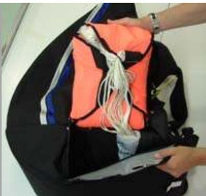
Place the deployment bag containing the reserve inside the reserve container of the harness, with the handle facing up as shown.
