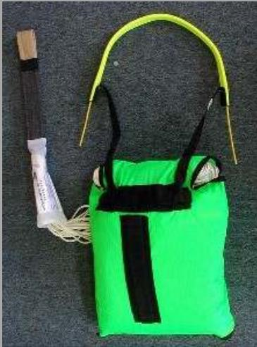
Your harness is supplied with a deployment handle fitted in the correct way. Remove the handle by pulling it out of the elastic retainers. Attach the handle to the deployment bag (44120T) supplied with your [Mayday](#) reserve parachute. If your Reserve is not already fitted inside the deployment bag, follow the instructions for doing this on the [Mayday](#) page.
