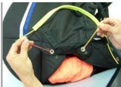
Now close flap No.1 and No.2 over the reserve and thread the two pull cords through the grommet on flap No.2 and close flap No.2 and No.3 over the reserve and thread the two pull cords through the grommet on flap No.3.
