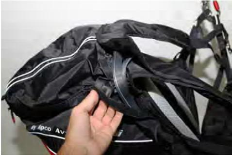
**Step 5:** Join the two bridles, pre attached to the harness and guide them through the Velcroed sleeve along the right side of the harness, up to the rescue pocket.
