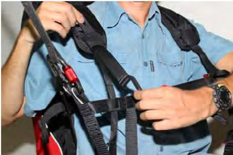
Shoulder Strap Adjusters are a pull-pull system. They are located at the end of the shoulder straps. The shoulder straps pass through the chest strap creating a "floating shoulder-seat system" for easier entry and exit into the harness during take off and landing.
