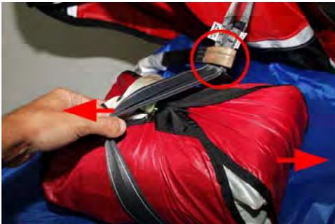
**Step 6:** Place the two big loops of the #42024 bridles together, attach the reserve parachute bridle to the center of the two #42024 bridles using a larks head knot.
