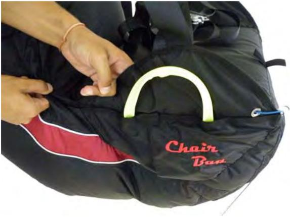
Pull out the speed system lines.
