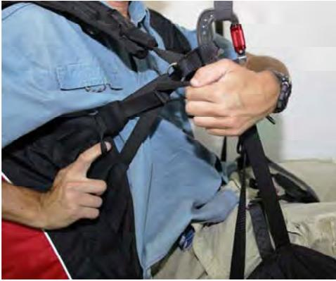
**Back Support Straps** are best adjusted while the harness is suspended from a suitable structure before flying for the first time. To change to full up right position, pull on the forward loop. To recline back, pull on the back loop.
