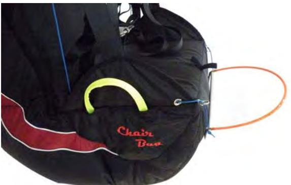
Re-connect the Brummel hooks to the speedbar lines as shown at the beginning.
