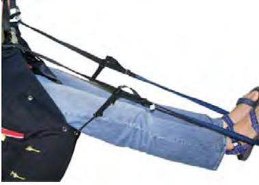
Is really useful for improving your aerodynamic shape, improving the weight shifting and taking the load off your feet. It also helps to push back in the harness without having to take your hands off the brakes.
