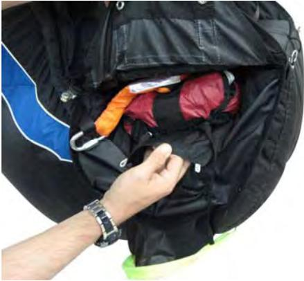
**Step 9:** pull the cloth tongue in between the attachment loops of the deployment handle.
