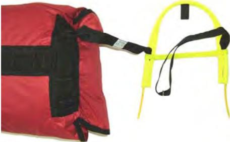
**Step 2:** Attach the handle to the deployment bag supplied with your reserve parachute. The handle has a split ring fixed to one of its attachment loops. Thread the first (without the Split Ring) attachment loop through one of the attachment points on the deployment bag. Pass the handle through the protruding loop to form a larks Head knot.
