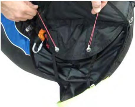
**Step 11:** thread the two pull cords through the upper closing flap grommets.
