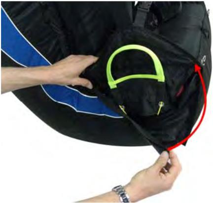
**Step 14:** neatly close the Y bridle sleeve (pressing the Velcro together) hold the lower flap corner and attach it by Velcro to the top flap front end.
