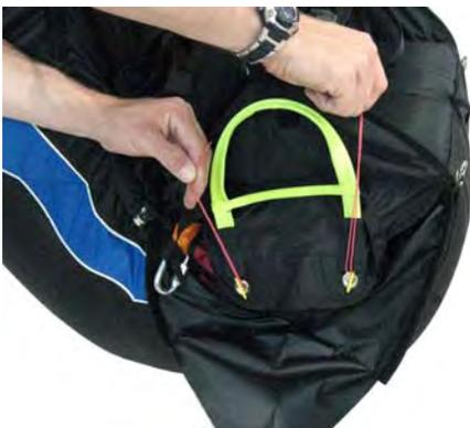
**Step 12:** fit the deployment handle in to the upper flap by pushing its ends (cable first) into the elasticized sleeves with the locking cables protruding on the other side. The webbing part of the handles should be pushed almost all the way into the elasticized sleeves (stop about 8-10mm before the opening where the cable is protruding). Pull the closing loop through the grommets and push the locking cable through it
