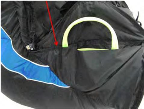
**Step 15:** neatly attach the left Velcro. As shown.
