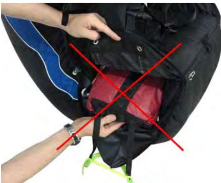
**WARNING! Do not place the reserve with handle attachment side facing upwards**
