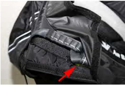
**Step 4:** Attach a #42024 Universal harness bridle to the reserve connection loop located on each shoulder strap of the harness **(THROUGH THE YELLOW WEBBING LOOP).**
