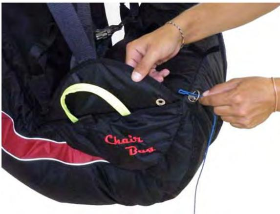
Pass the speed system lines through the bungee-secured metal rings at the front of the seat
