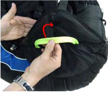
**Step 17:** secure the deployment handle to the harness using the Velcro As shown.
