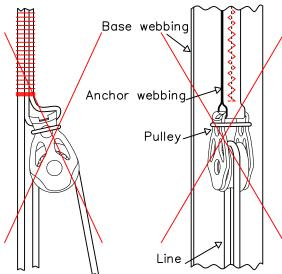
Stitching the anchor webbing to the base webbing all the way will fix pulley rigidly preventing flexing on pulley to follow the line direction.
