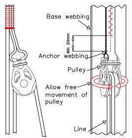
Do not stitch the anchor webbing to the base webbing all the way. Leave minimum 20mm—30mm free to allow twisting of pulley to follow the line direction.
