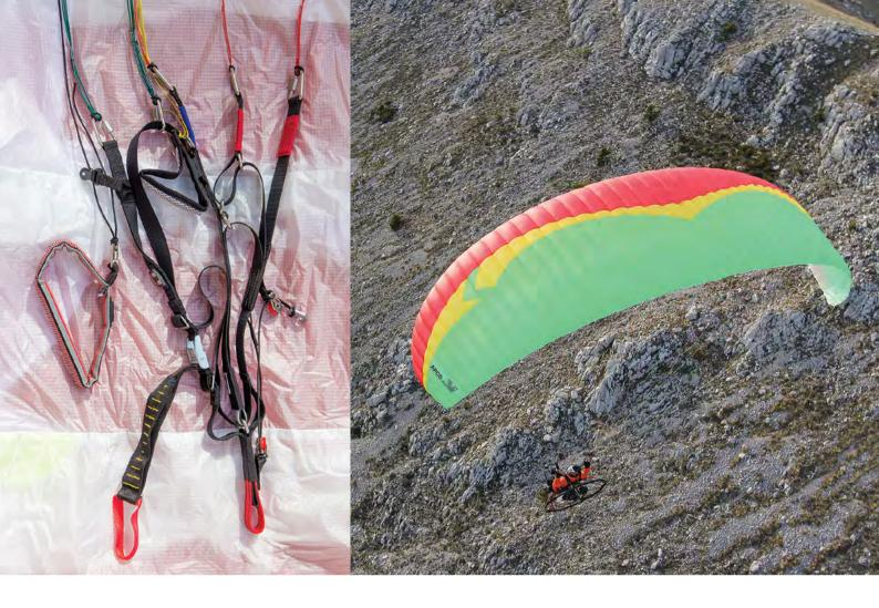
The wing is made from Gelvenor cloth with a silicone coating on the front half. This should mean the wing stands up well to general use and being dragged around as you hone your ground-handling skills. All the lines are sheathed, which makes for easy handling on the ground and in the air. They are all nicely colour-coded too, making it easier to find the line you want.
