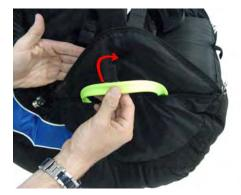
**Step 17:** secure the deployment handle to the harness using the Velcro As shown.
