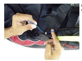
Pass the speed system lines through the pulley on either side of the harness.
