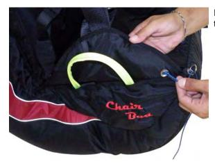
Feed the speed system lines through grommets located at the front of the harness.
