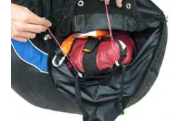
**Step 10:** Individually thread two pull cords through the two closing loops located on the cloth tongue (one through each loop). The pull cords must be between the attachment loops of the deployment handle.
