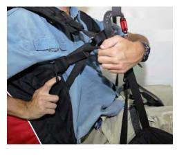
Back Support Straps are best adjusted while the harness is suspended from a suitable structure before flying for the first time. To change to full up right position, pull on the forward loop. To recline back, pull on the back loop.
