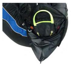
**Step 13:** Carefully remove the pull cords by passing one of its ends under the locking cable and pulling it out slowly.
