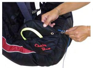
Pass the speed system lines through the bungee-secured metal rings at the front of the seat
