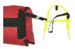
**Step 2:** Attach the handle to the deployment bag supplied with your reserve parachute. The handle has a split ring fixed to one of its attachment loops. Thread the first (without the Split Ring) attachment loop through one of the attachment points on the deployment bag. Pass the handle through the protruding loop to form a larks Head knot.
