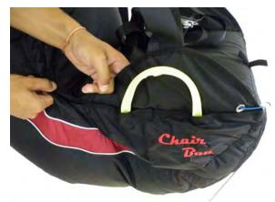
Pull out the speed system lines.
