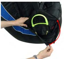
**Step 14:** neatly close the Y bridle sleeve (pressing the Velcro together) hold the lower flap corner and attach it by Velcro to the top flap front end.
