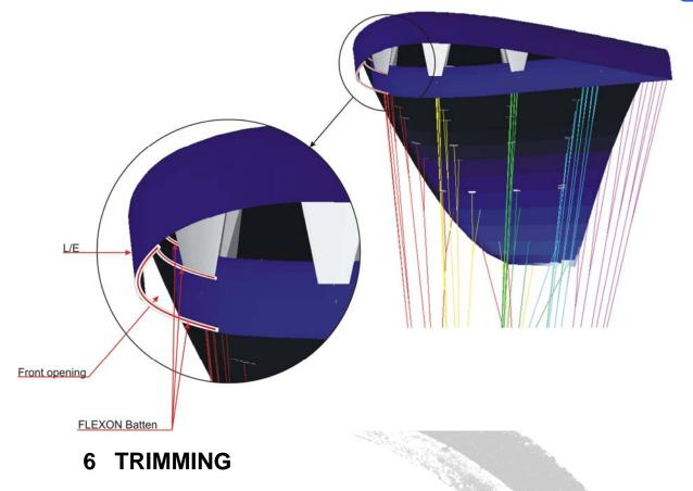
All Apco gliders are trimmed for optimum performance combined with unsurpassed safety. It is very important not to re-trim or tamper with any of the lines or risers as this may alter the performance and safety. Trimming of the brake line should be done in accordance with this manual and carefully checked before flying.
