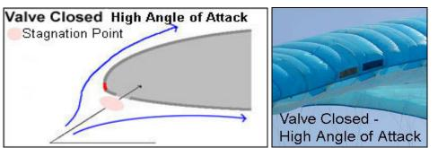
The LIFT 400/450 is equipped with an Active HIT Valve system (patent pending) to improve the overall performance and safety of the wing especially during accelerated flight.
