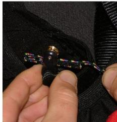
5. Thread the line through your harness pulley system. Sometimes the loop is hard to get through the pulleys. When it is threaded through, reverse steps 2 to 4 to reconnect the brummel hooks.
