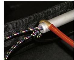
6. The length of the lines is adjusted by moving the knot where it stops against the end of the bar. Make sure you don't set it overtight so that the accelerator system is being applied before pushing the bar.
