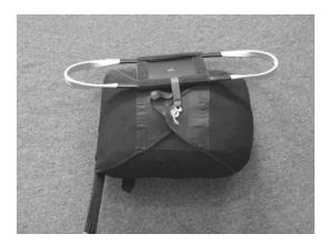
**6.** Finally attach the deployment handle to the container by placing the handle on the Velcro attachment located on the front of the container.
