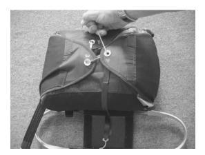
**5.** Lock the container by pulling the loop through the last eyelet with the pull cord and pass the curved locking pin through the closing loop. Carefully remove the pull cord by slipping it under the pin and pull it out slowly so as not to damage or burn the closing loop.
