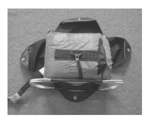
3. Thread a pull cord through the closing loop located on flap #1
