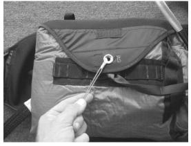
**4.** Thread the pull cord through each grommet (eyelet) Located on each flap according to their order (2, 3, 4).
