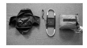
1. Attach the handle (supplied with the p/m container) to the deployment bag containing your parachute. To do this thread the attachment strap through the center Loop formed by the webbing straps on the deployment bag.
