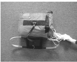
**2.** Lay the outer container on the table as shown, Place the inner container on top of it so that the bridle loop now protrudes from under the inner container and the deployment handle attachment strap is on top as shown.
