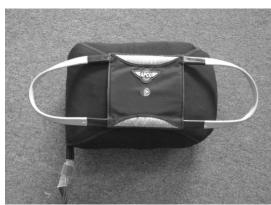
Before each flight it is highly recommended to verify that the locking pin is secure in its place using the transparent plastic window.
