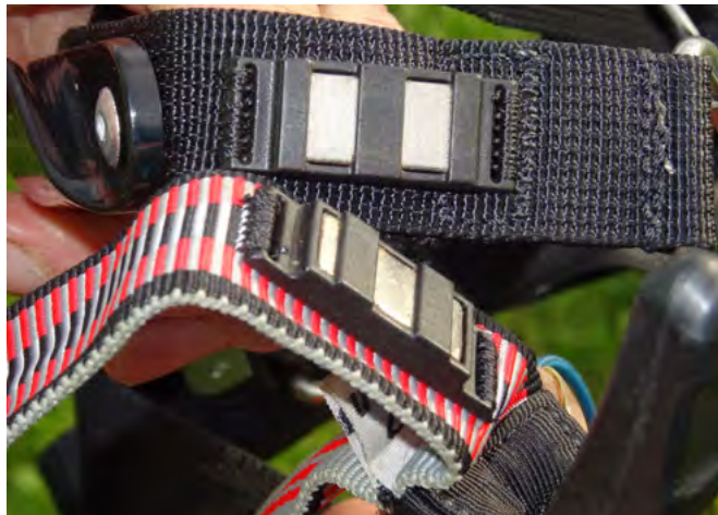
Clever: the shape of the magnets puts the handles automatically parallel with the riser, no matter what angle they are put.
