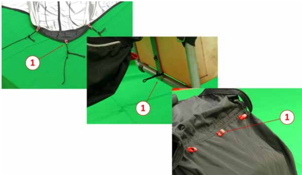
Photo C: Point 1 connects middle bottom of the pod to the middle of the PM frame, or optionally it could be connected to loops at rear middle bottom of the harness.
