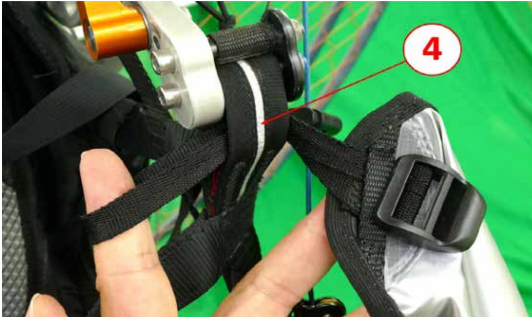
Photo M: Points 4 (left and right) (see also Photo A ) – are connected to the hookup points of the harness.
