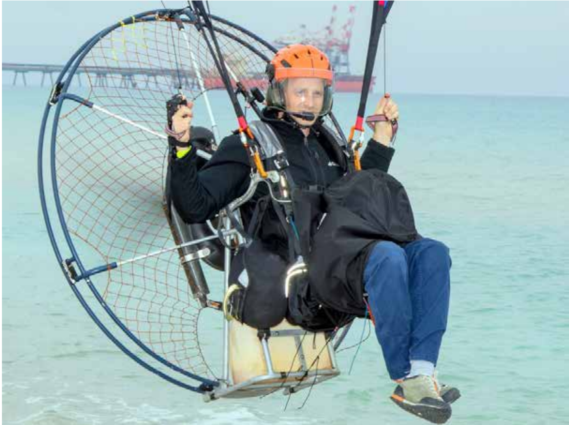
Photo T: Pilot's legs and the Pod position after take-off and before landing.
