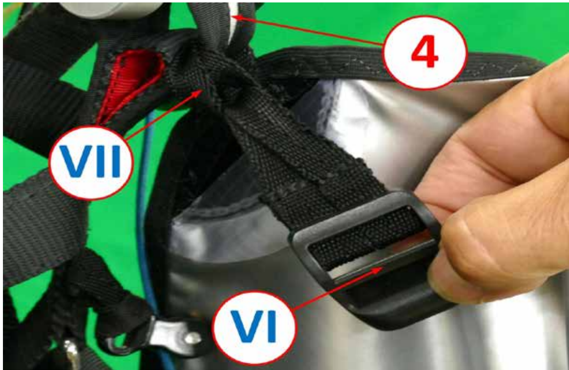
Photo Q: Then, pass VI (the ladder-lock slider) through its own webbing loop, and tighten the knot against the harness.
