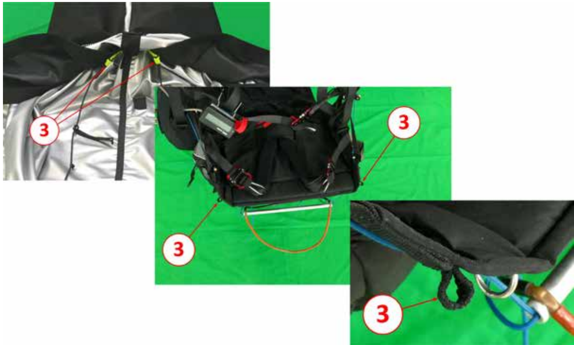
Photo E: Points no 3 (left and right), yellow webbing loops on the Pod – assembled to points no 3 on the harness by a long adjustment line, with prepositioned knots. On harnesses which do not have these connection points, you can connect to the front flap webbing or speed system pulley attachments.
