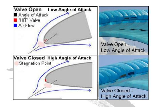
The LIFT 400/450 is equipped with an Active HIT Valve system (patent pending) to improve the overall performance and safety of the wing especially during accelerated flight.
