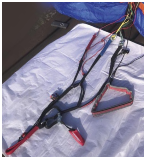
Paramotor riser setup - note trimmer and neat V-link connectors
