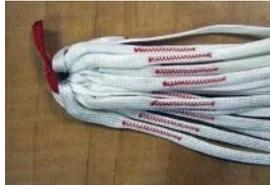
Spliced line connection detail
