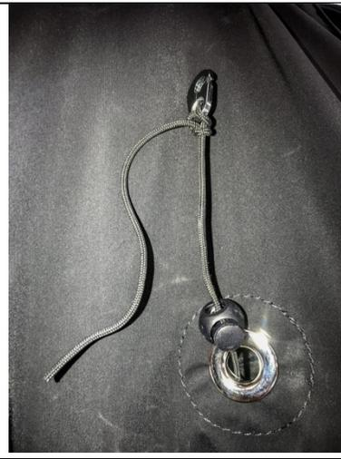
Cord-lock and Brummel hook on the Speed bar line where it exits the skirt through the eyelet.
