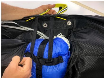
Place the reserve in the container with the handle attachments to the lower side as shown. In this way, the handle straps will help to open the zippers immediately. The reserve bridle should be under the reserve, and exiting into the zipped bridle sleeve, which can be closed later in the sequence.
