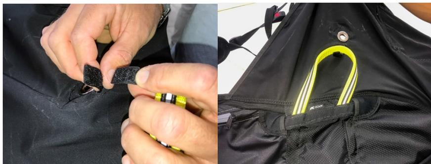
Attach the Velcro keeper on the handle to the matching velcro tab on the side of the harness next to the speed bar exit eyelet, and finally close the bridle cover zip by bringing the zipper toggle all the way down from the shoulder to the container, and back up again to close the zip, and stow the zipper toggle in the provided pocket on the shoulder at the end of the zipper.
