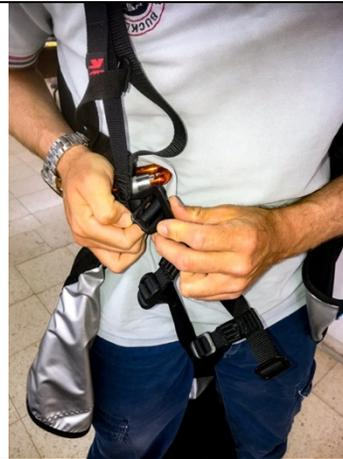
Insert the corresponding buckles into the female parts next to the carabiners
