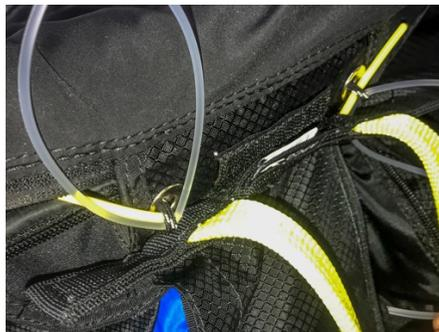
Close the reserve container flap using the two locking loops passed through the eyelets, and locked using the yellow cables on the reserve handle. The handle straps should be routed between the two locks.
