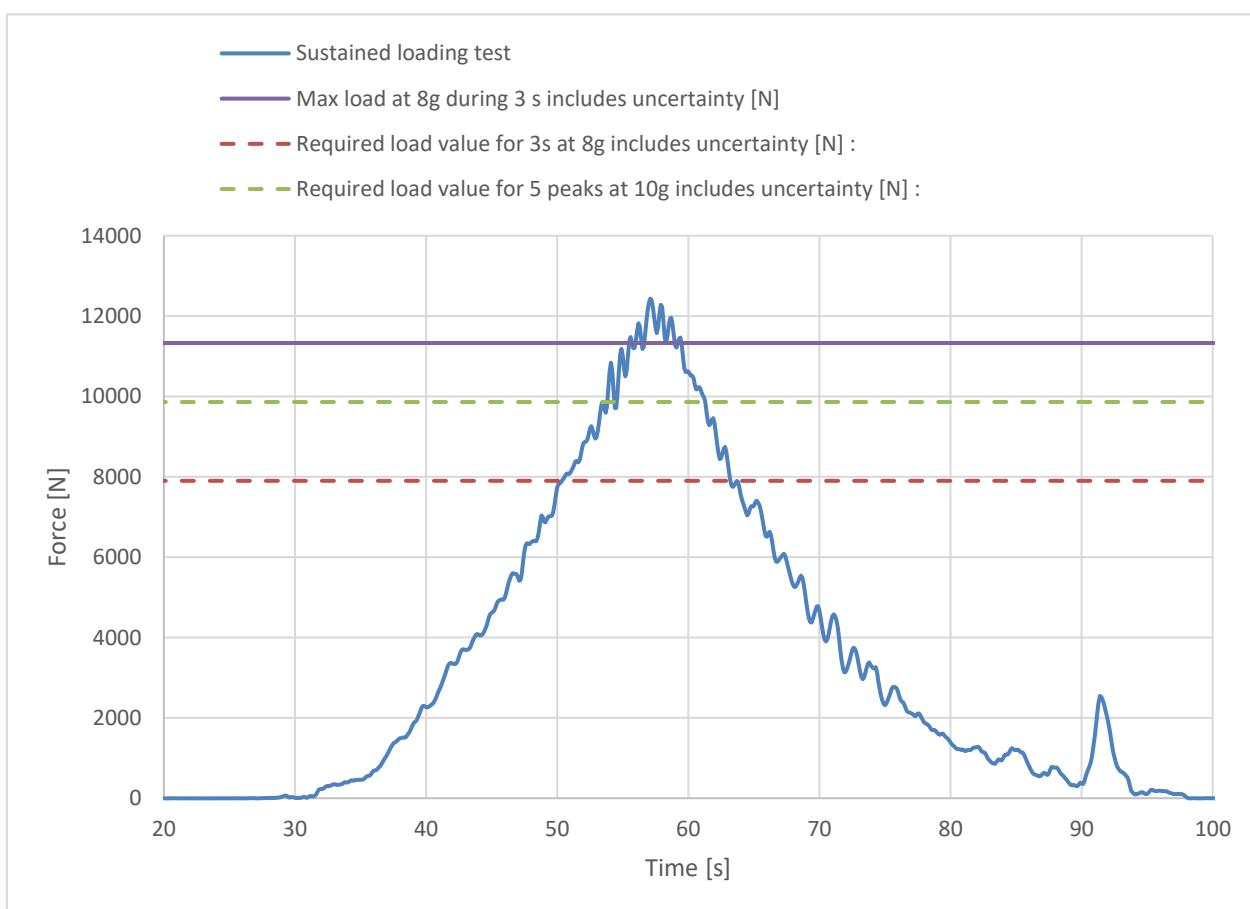
**Sustained loading test results<sup>(3)</sup>**Result : **POSITIVE**Calculated max load value with 3 sec or five peaks [kg] : **144.38**
