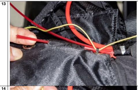
Lock the first of the three main closures also using the short locking "pin", and then pass it under the sleeve.
