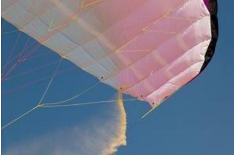
Fig. 10 – Butt Hole II valve at trailing edge
