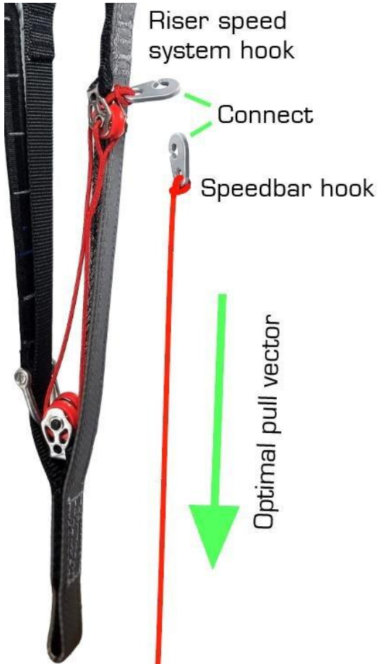
Fig. 6 – Speed system: Riser speed system hook connects to Speedbar hook; green arrow shows optimal pull vector
