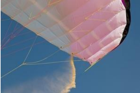
Fig. 10 – Butt Hole II valve at trailing edge
